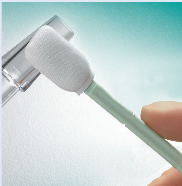
Figure 1. A polyester knit swab used for surface sampling. A notched handle allows for easy snapping the swab head into the vial.
